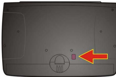
**Figure 2-14 Infrared Port - COM2 Port**
