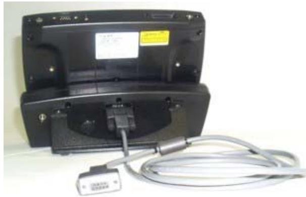
**Figure 2-15 ActiveSync Cable Connected to Serial port on Cradle**
