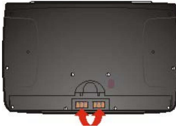
**Figure 1-4 MX3X Battery Contacts**
