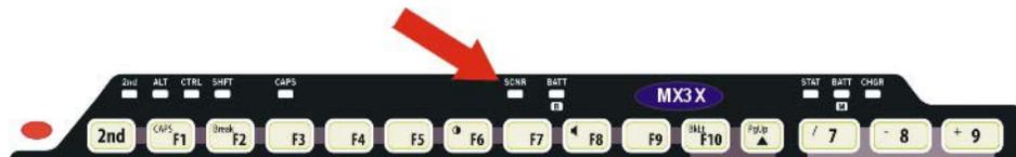
**Figure 1-17 Scanner LED Location**
