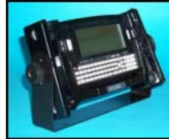
**Figure 2-15 Vehicle Mounted Cradle**
