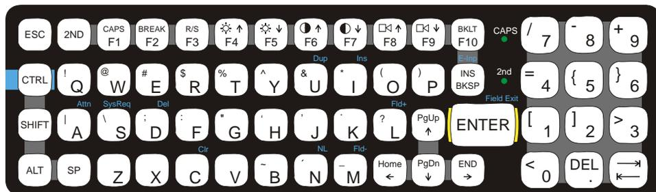
**Figure 2-32 IBM 5250 Specific Keypad**
