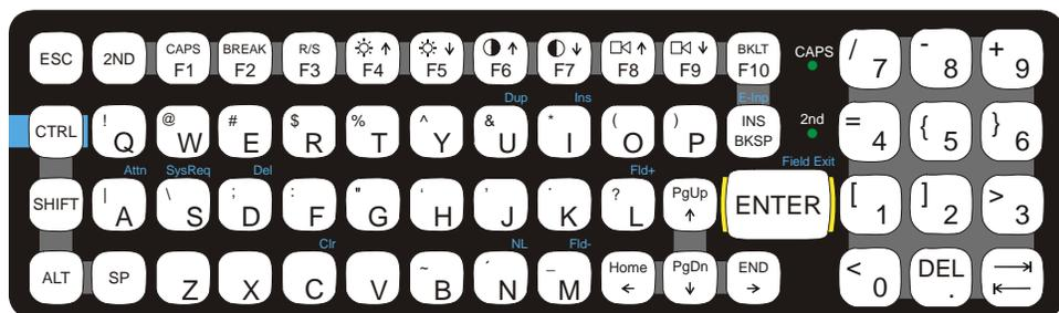
**Figure A-4 IBM 5250 Specific Keypad**
