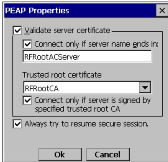
**Figure 5-57 PEAP Properties, Connect Only If Server Name Ends In**
