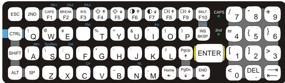
**Figure A-3 IBM 3270 Specific Keypad**
