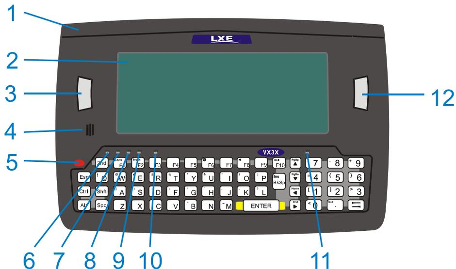
**Figure 1-2 VX3X Components, Front View**
