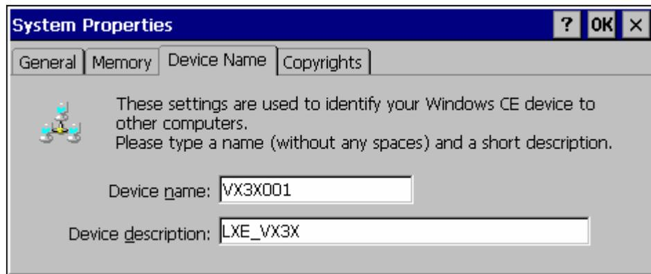
**Figure 3-29 System / Device Name**
