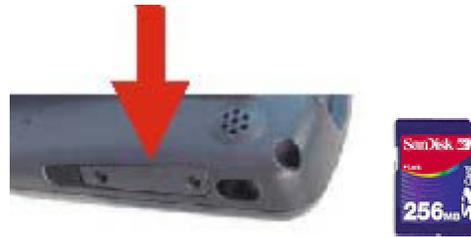
**Figure 3-2 Secure Digital Memory Interface Card Location**
