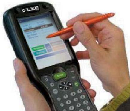
**Figure 1-6 Tapping with the Stylus**
