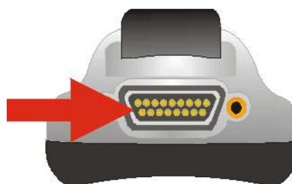
**Figure 4 RS-232/USB Communications and Charging Port**
