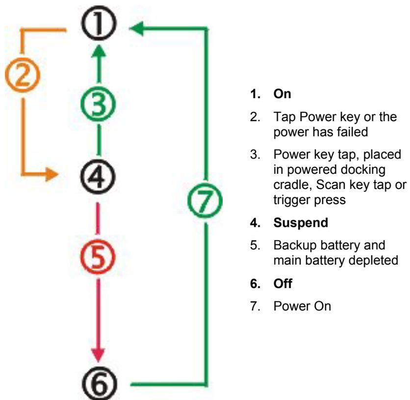
**Figure 19 Power Modes – On, Suspend and Off**
