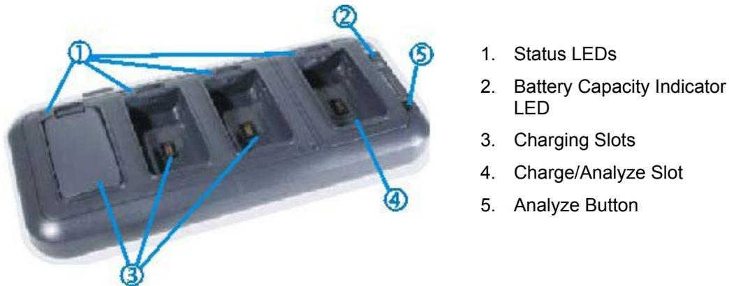
**Figure 20 Multicharger / Analyzer**
