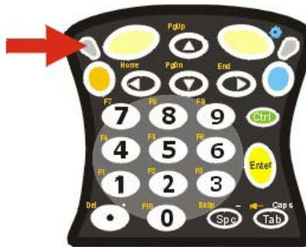
**Figure 1-9 Battery Charging LED**
