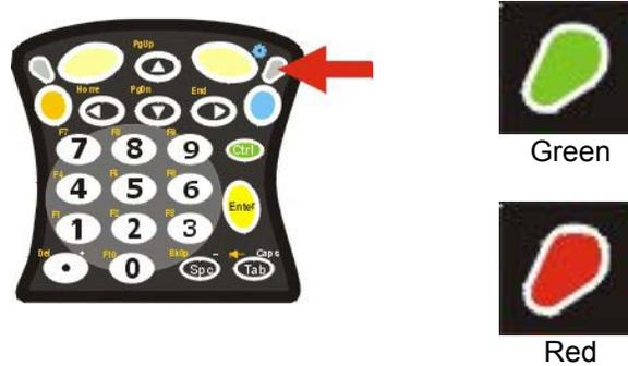
**Figure 1-16 Scanner LED Location**
