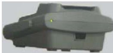
**Enhanced Desktop Cradle** requires AC power before Main Battery charging can commence. It will charge both the main battery in the MX5 and another Main Battery at the same time.
