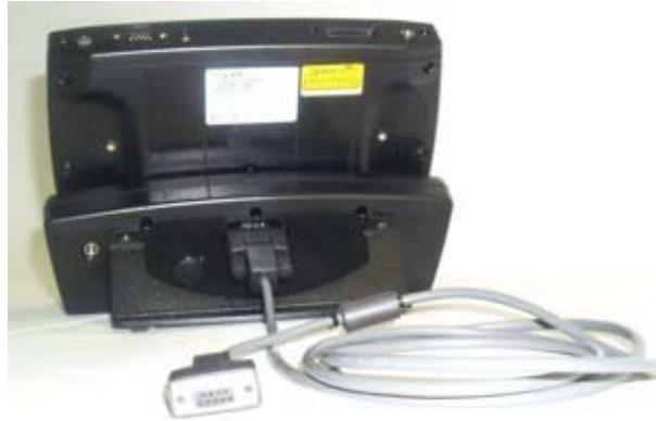
**Figure 27 ActiveSync Cable Connected to Serial port on Cradle**
