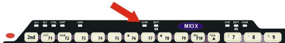
**Figure 14 Scanner LED Location**
