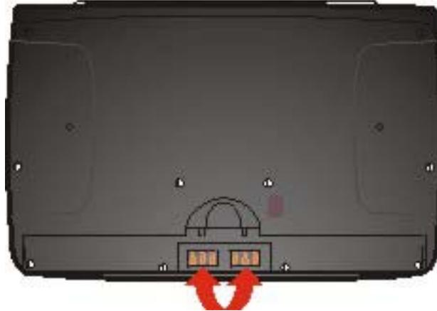
**Figure 6 MX3X Battery Contacts**
