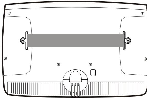
**Figure 1-8 MX3-CE With Handstrap Installed**
