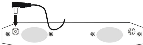
**Figure 1-12 Connect External Power Supply**
