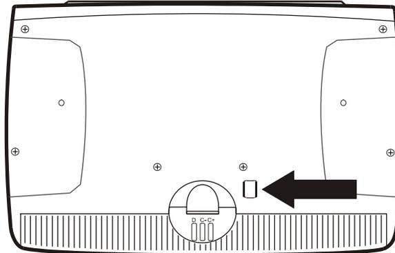
**Figure 2-13 Infrared Port - COM2 Port**
