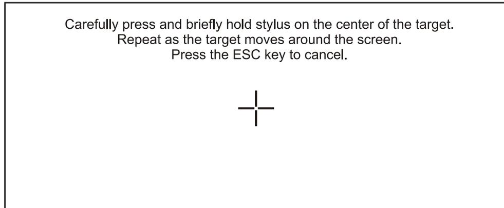
**Figure 1-14 Touch Screen Recalibration**
