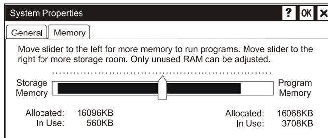
**Figure 4-21 System Properties / Memory Tab**
