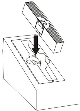
**Figure 3-3 Insert Main Battery in Charge Pocket**
