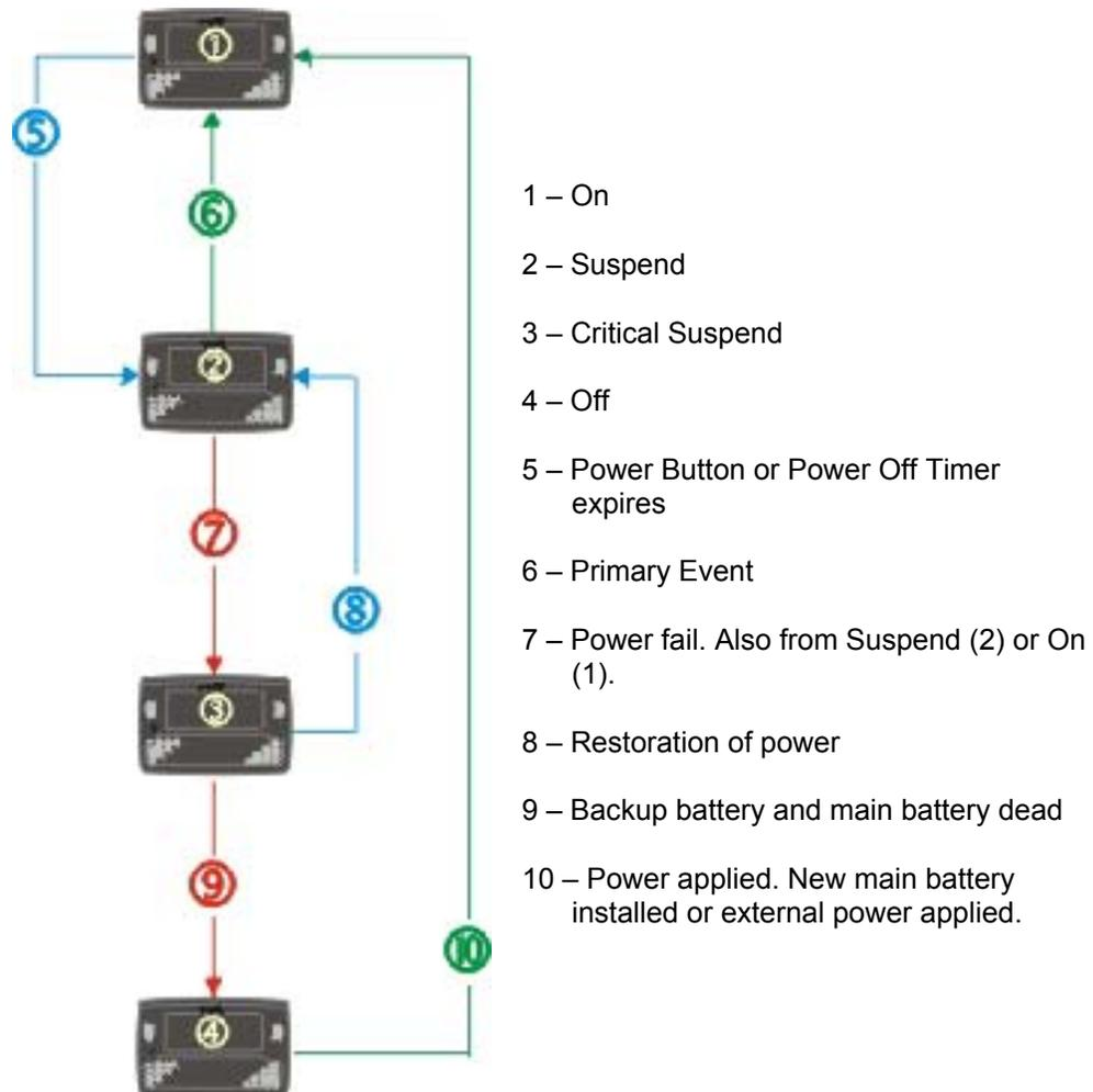
**Figure 1-23 Power Modes – On, Suspend, Critical Suspend and Off**
