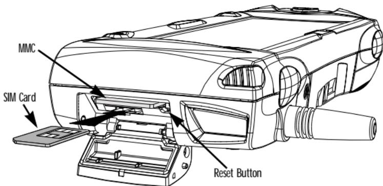
Figure 2.11 Reset Button Location
