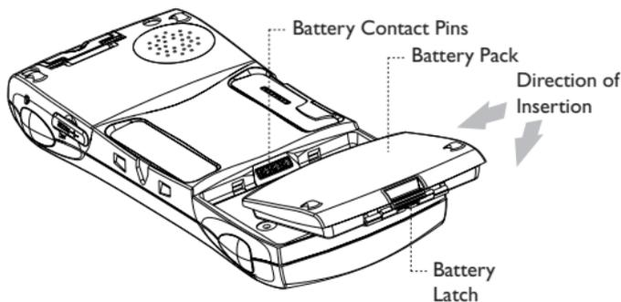
Figure 2.6 Battery Insertion
