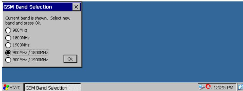
5. Select the correct band setting for your GSM provider. Then click on the **OK** button. The hourglass will appear. When it is gone, use the **X** button to close *GSM Band Selection*.
