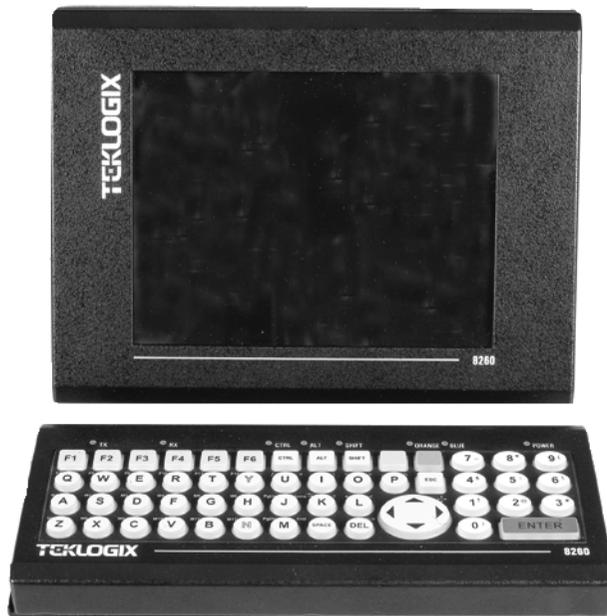
Figure I.8 The 8260 Vehicle-Mount
