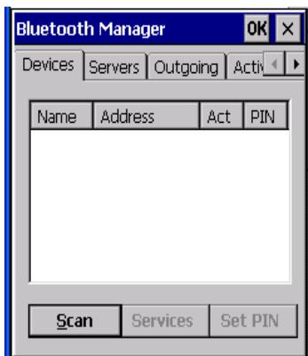
If you intend to pair devices (a headset, for example), power on and bring the devices within 5 m (16.4 ft.) of the hand-held before proceeding with the discovery process described below.
